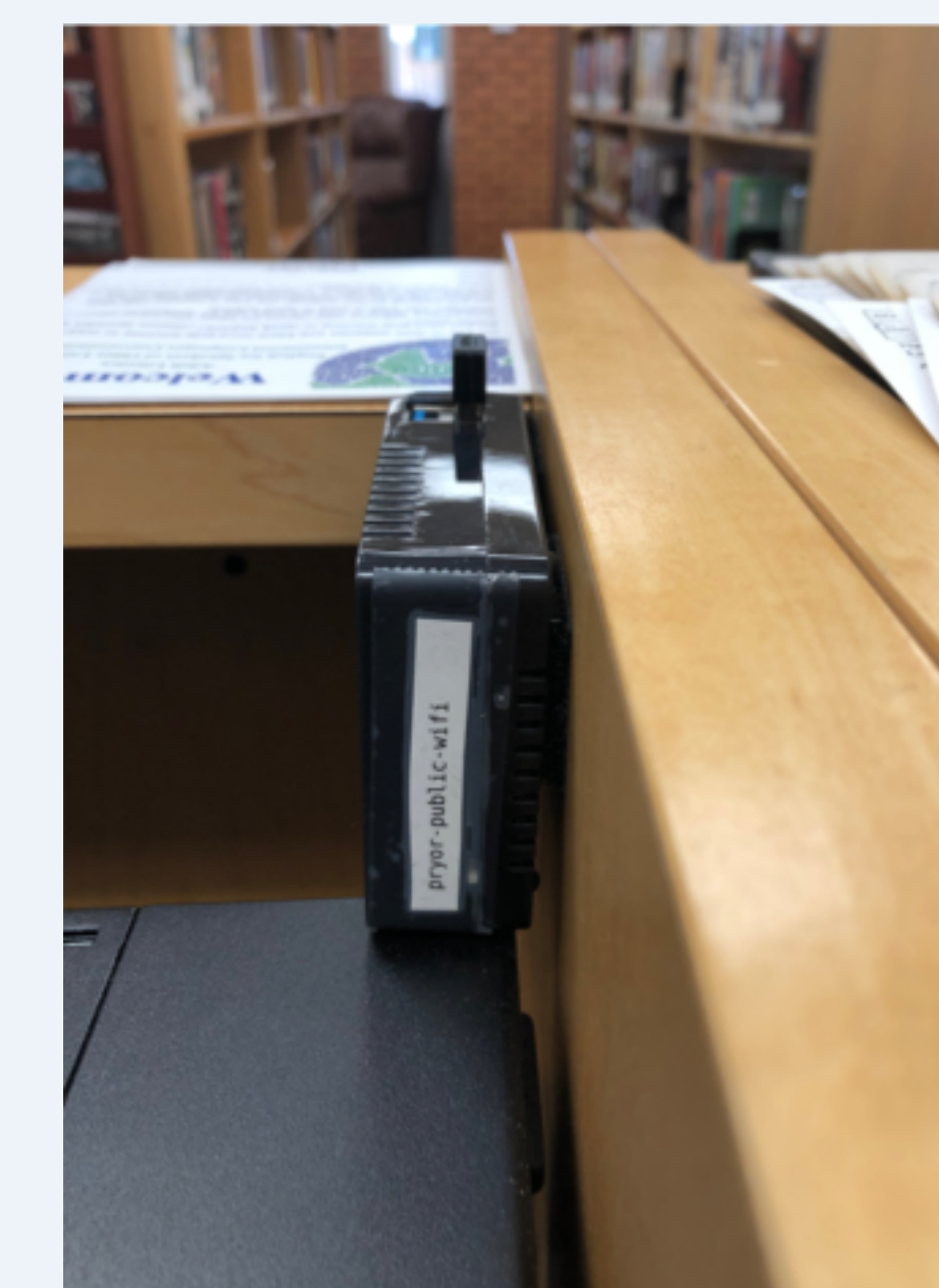
Photo left of Odroid XU4 broadband measurement device installed at the Pryor Public Library in Oklahoma
